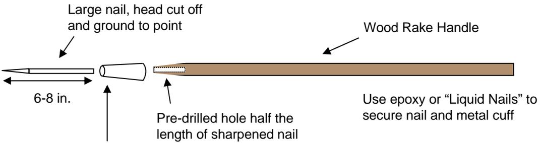
Large nail, head cut off and ground to point
